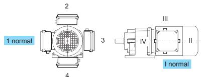
Cable entries at brake- motors only possible at pos. I and III.
